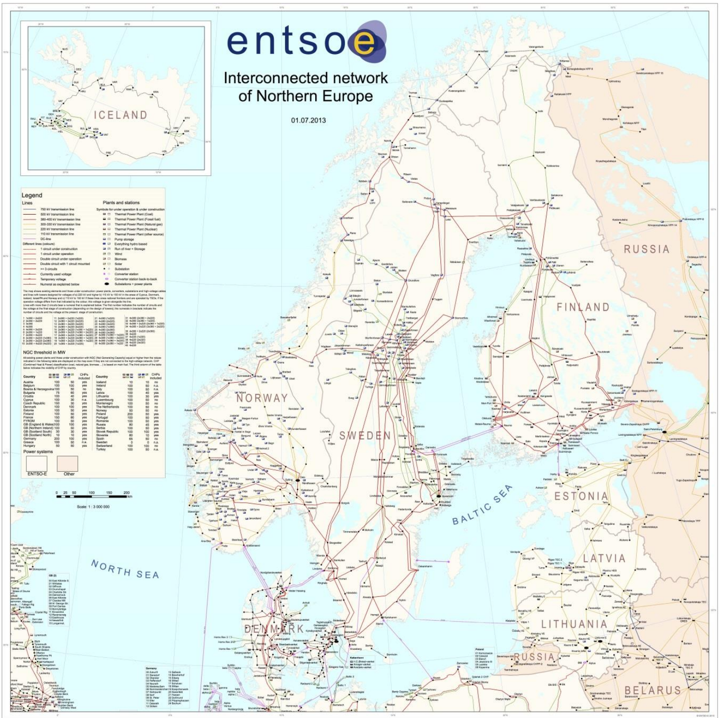
FIGURE 1.3.1 THE NORDIC MAIN GRID [2]
