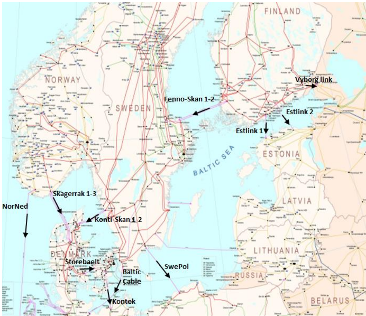
FIGURE 2.1 PART OF THE NORDIC GRID MAP SHOWING THE HVDC LINKS. THE ARROW INDICATES THE DIRECTION OF EXPORT
