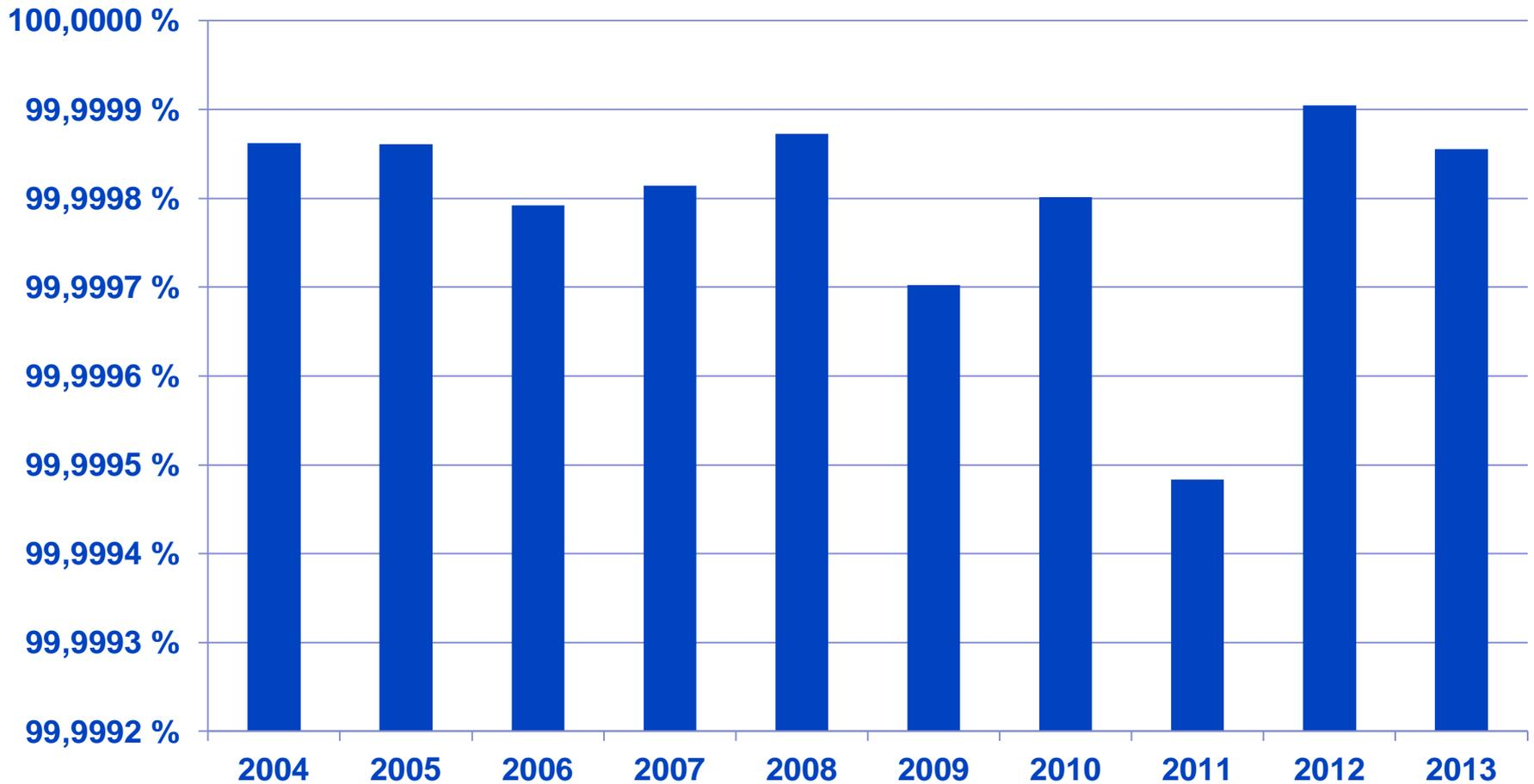
Transmission reliability = energy supplied / (energy supplied + energy not supplied due to disturbances)
