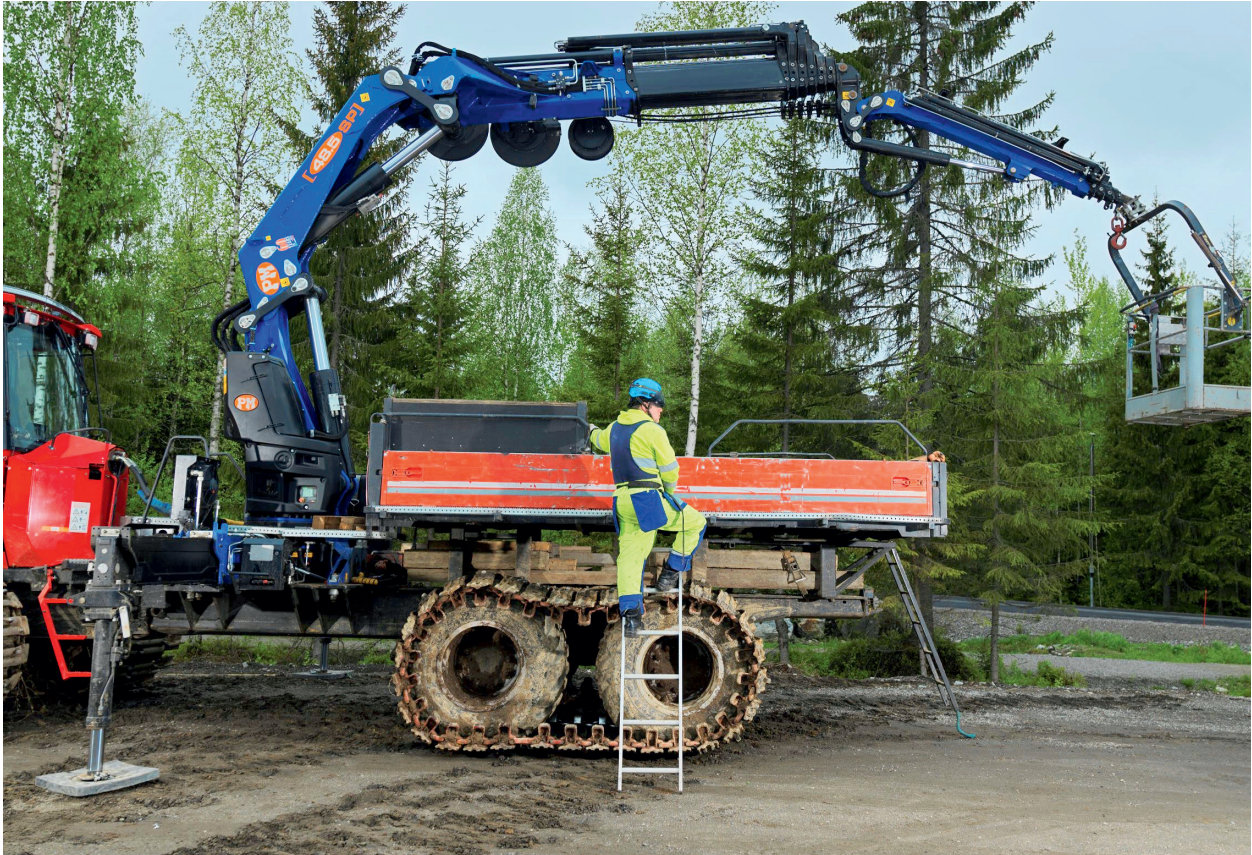
Access routes to forest machinery were improved by adding ladder and step solutions, access bridges and handrails.
