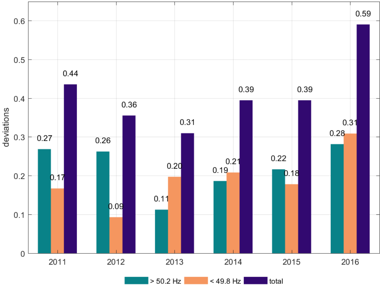
Figure 3.50. Daily average number of frequency deviations larger than \pm 200 mHz for years 2008-2016
