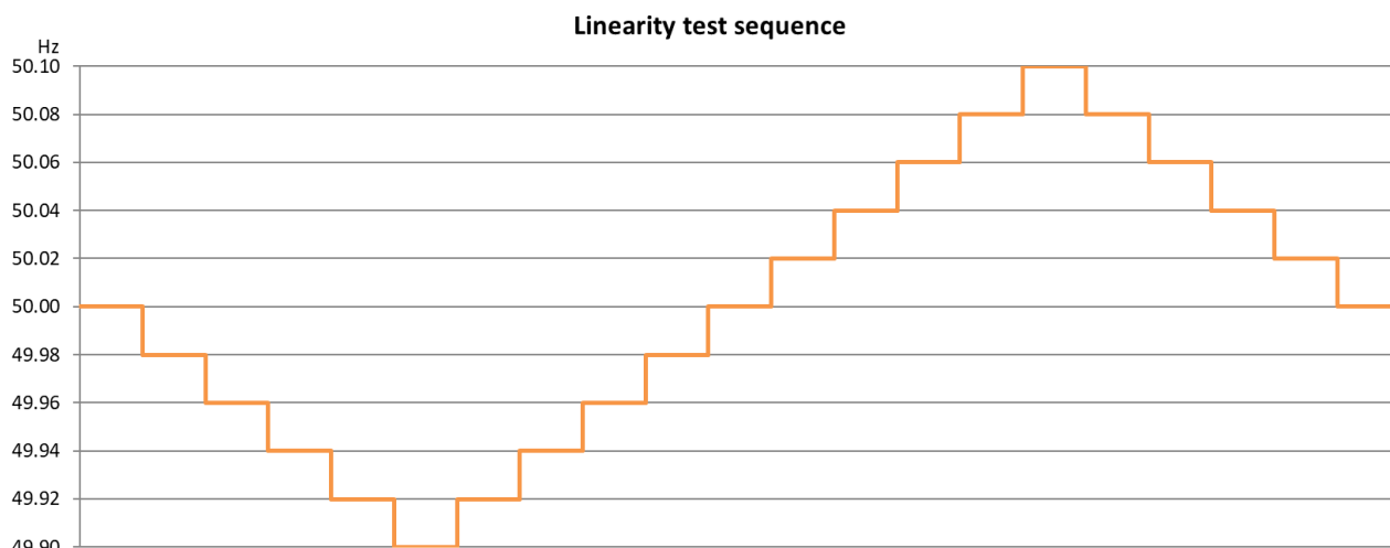
Figure 13. Grid frequency test signal for the FCR-N linearity test for non-continuously controlled reserves.
