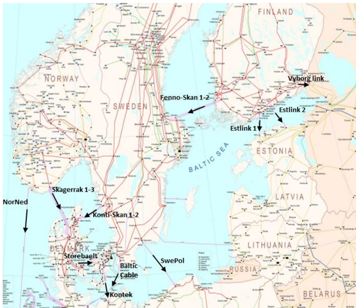
FIGURE 7.19 PART OF THE NORDIC GRID MAP SHOWING THE HVDC LINKS. THE ARROW INDICATES THE DIRECTION OF EXPORT.
