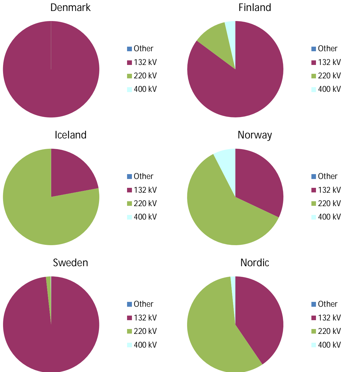
FIGURE 4.1A ENERGY NOT SUPPLIED (ENS) IN TERMS OF THE VOLTAGE LEVEL OF THE INITIATING FAULT IN 2012.
